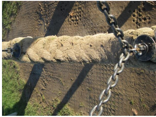
Fig.5(c). Fraying rope.
