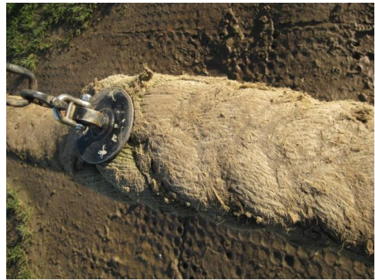
Fig.5(b). Fraying rope.
