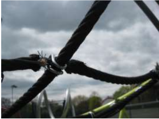
Fig.5(c). Worn climbing net.
